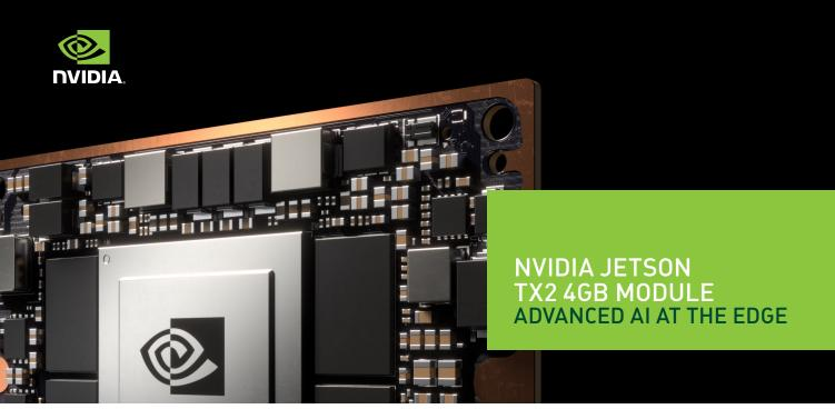
The NVIDIA® Jetson™ TX2 4GB module delivers powerful computing performance in a small credit card form factor to run modern AI workloads. It can be configured to operate between 7.5 W and 15 W, making it ideal for a diverse set of intelligent edge devices like robots, drones, smart cameras, and portable medical devices. The module offers three times the performance per-watt of Jetson Nano, enabling the development of high-performance, energy-efficient, and affordable products.
